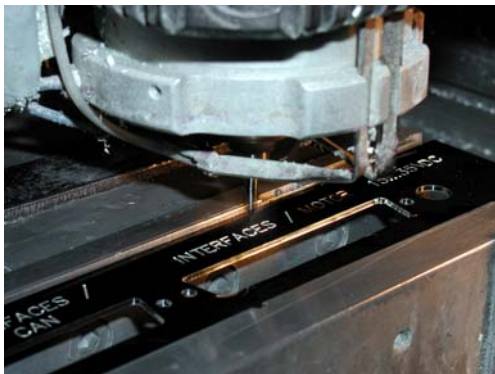
Fig.8 CNC front panel manufacturing
