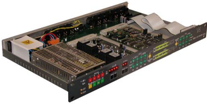
Fig.4 19"/1RU frame AES/EBU shuffler
