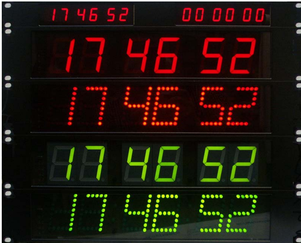
Fig.1 RTC/LTC Time Code 19" Displays LTCD119/219-R(red)/G(green)
